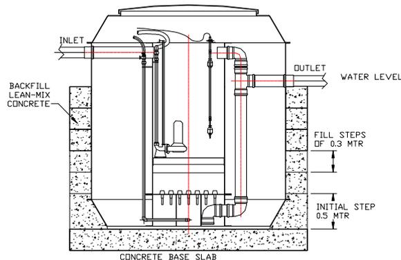
Step 9 Continue to fill with water and backfill to the rim of the tank.
